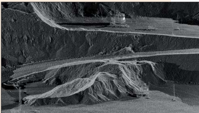
Fig.2 Automatic filtering of artificial objects
