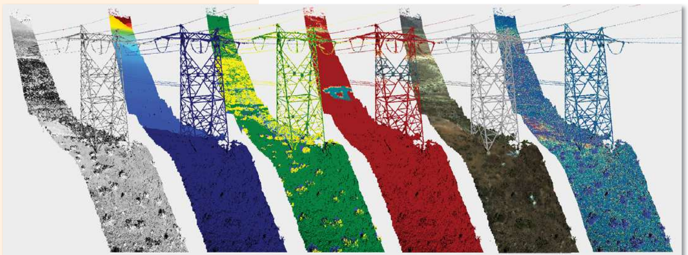
Fig. 3 Data visualized by (from left to right) reflectance, target range, multiple echoes ID, MTA confidence, true color, and pulse shape deviation
