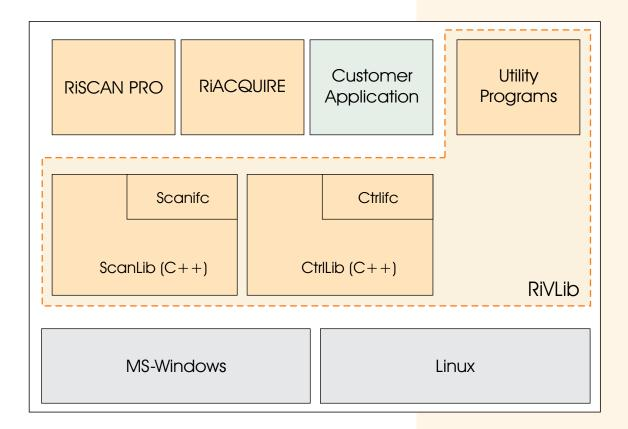
From a programmer's perspective RiVLib is a library that sits between application code and the operating system. Linux as well as Windows  $^{\circ}$  are supported.
