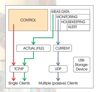
RIEGL V-Line scanners are equipped with a versatile data access system. The data connection can be made to the command and configuration interface (CONTROL), to the main measurement data stream (MEAS DATA), and / or to the so-called monitoring data stream (MONITORING), which consists only of a fraction of the measurement data and is intended to be used for monitoring the data acquisition by an operator in real time.
