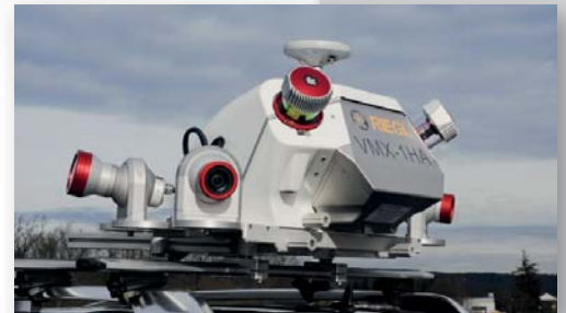
RIEGL VMX-1HA with (2x) 5 MP and (2x) 9 MP cameras
