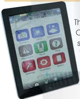
The system provides a number of useful **features** that help to make the user experience better overall. Operation of the *RIEGL VZ-400i* is easy with the integrated **Graphical User Interface (GUI)** via touch-screen, or by remote control of the scanner via VNC Viewer with any tablet PC or mobile device using Wi-Fi connection.
