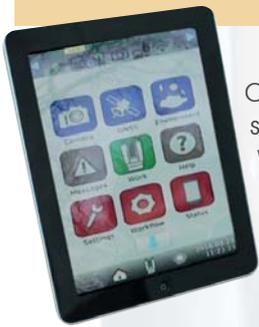
Operation of the *RIEGL VZ-400i* is easy with the integrated **Graphical User Interface (GUI)** via touch-screen, or by remote control of the scanner via VNC Viewer with any tablet PC or mobile device using Wi-Fi connection.
